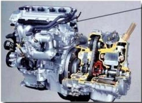
ICE (Internal Combustion Engine)
