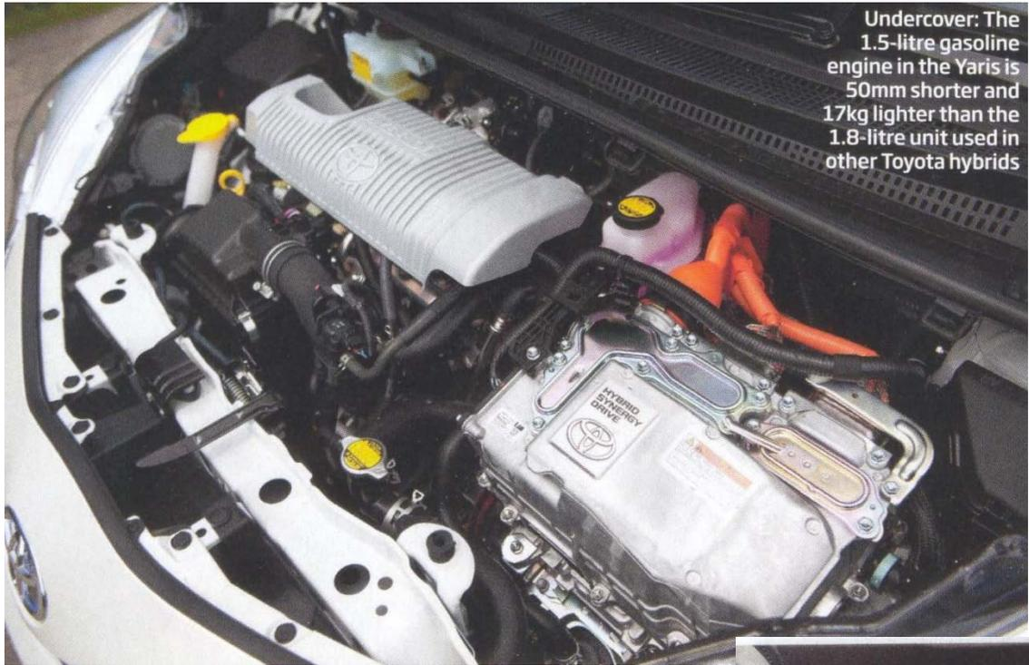
Undercover: The 1.5-litre gasoline engine in the Yaris is 50mm shorter and 17kg lighter than the 1.8-litre unit used in other Toyota hybrids
