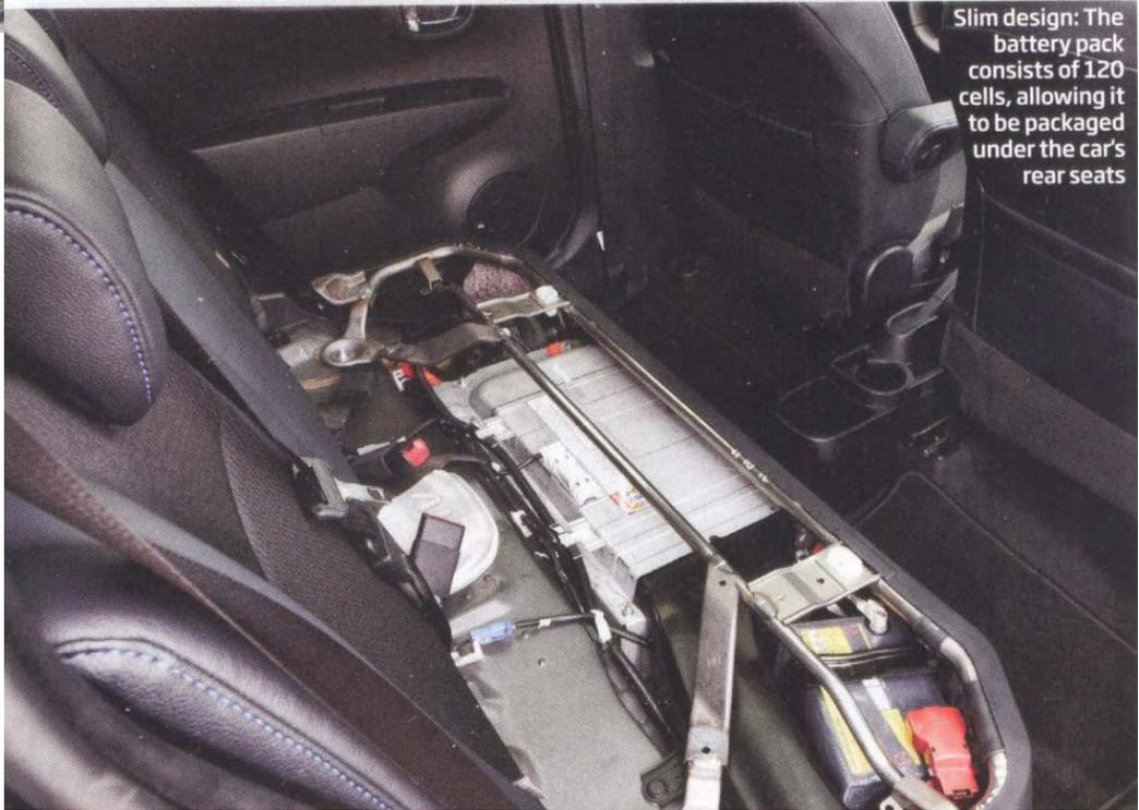
Slim design: The battery pack consists of 120 cells, allowing it to be packaged under the car's rear seats
